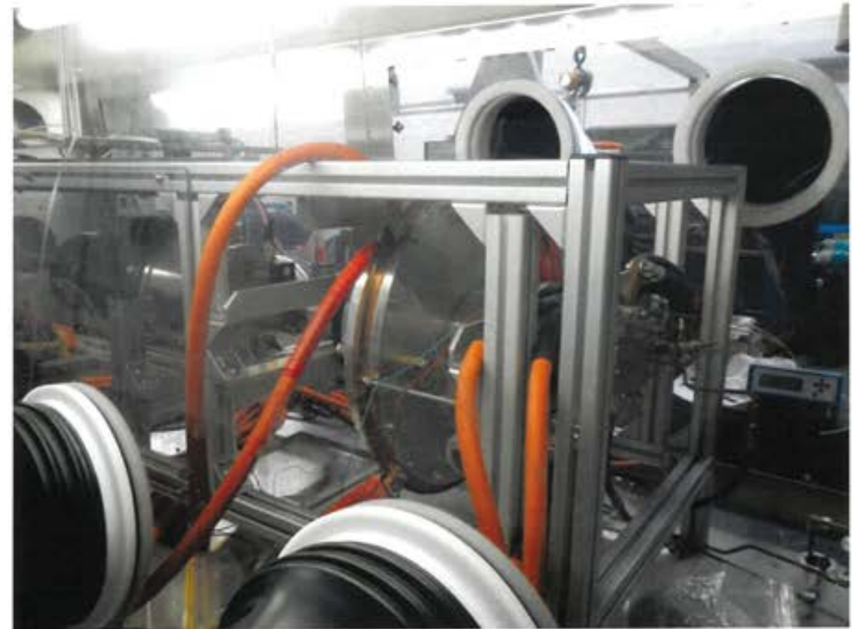
Large 400 mm outer disk (rotor of homopolar motor).
