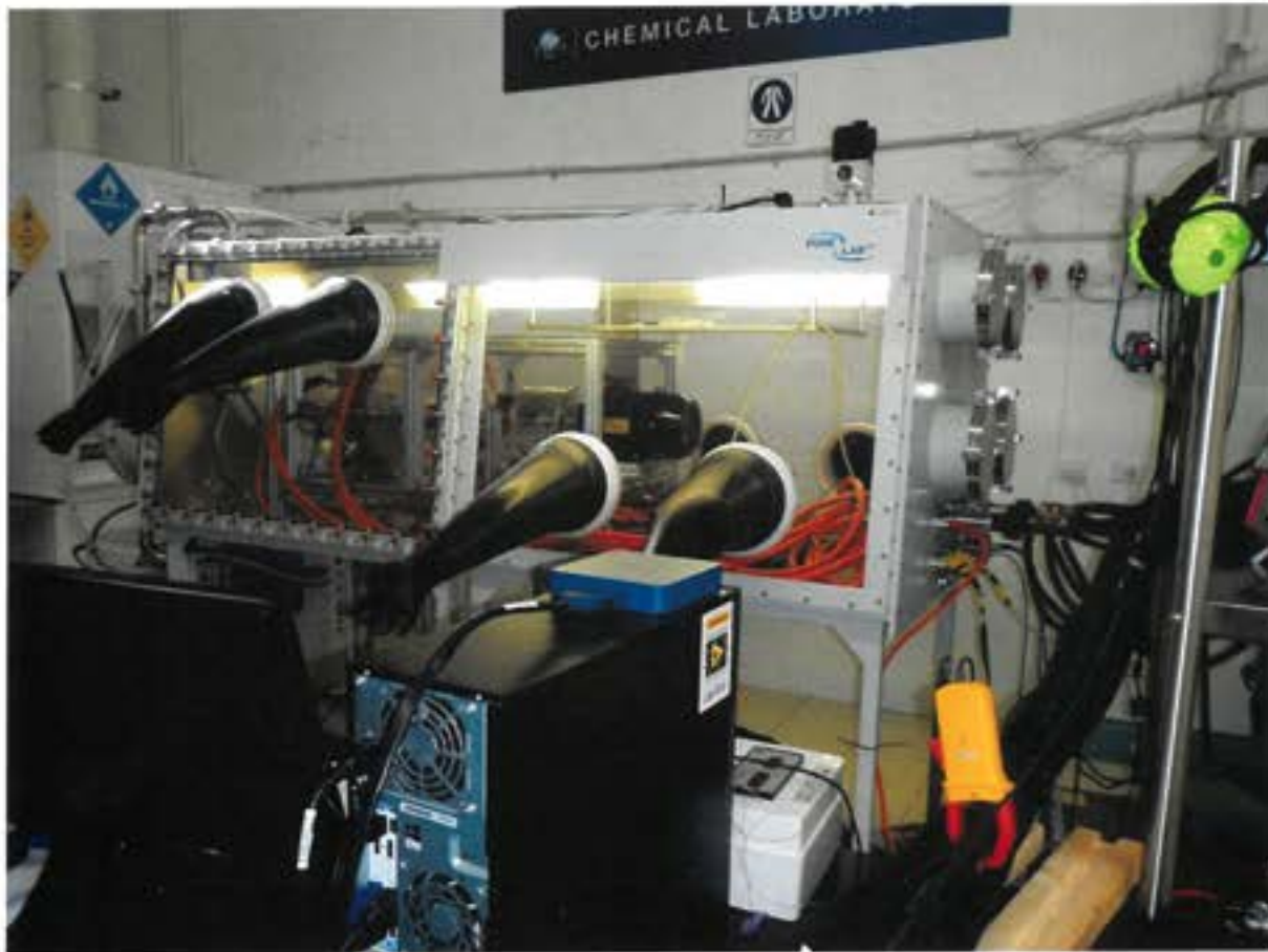
Argon gas glove-box for experimentation with LMCC
